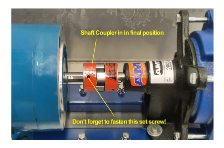
Once the water pump motor is verified to be running in a clockwise motion (same as the arrow indicator), the shaft coupler can be re-attached, and the set screw fastened to secure it in place.
